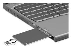
To remove the SmartC ard press the SmartC ard eject button (a) and remove the SmartC ard (b) as shown in the illustration below.
